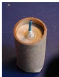
Place the end disc with the fuse, hot melt side up, in the casing. Tap the casing and press the end disc firmly on the contents. This will make the shell a little more rigid and resist the 'kick' from the launch better.
